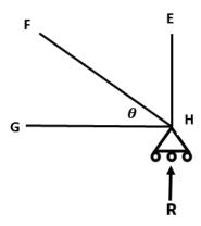
The roller joint has a reaction R of 35 kN. The compressive force in member GH is 12 kN and  $\theta$  is 40°.
