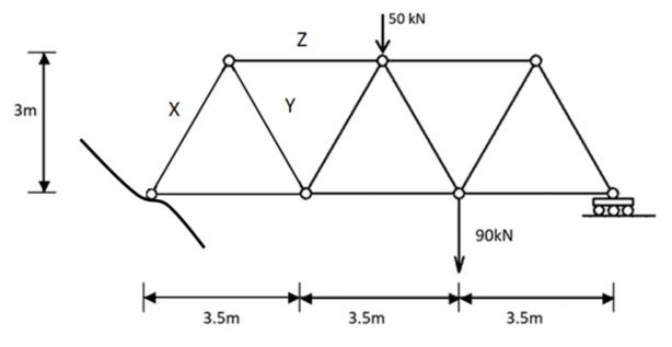
Calculate the forces in members X, Y and Z and identify whether the members are in tension or compression. Include a force diagram to support your response.
