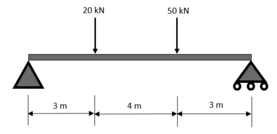
Draw shear force and bending moment diagrams for the beam. Show your calculations. Assume that the beam is without mass.
