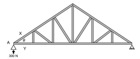
The truss is in static equilibrium. The reaction force  $R_A$  at support A is 300 N and  $\theta$  is 30°. Calculate the force in members X and Y and identify whether the members are in tension or compression. Include a force diagram to support your response.
