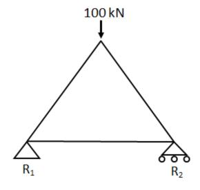
Calculate the reaction at supports  $R_1$  and  $R_2$ . The length of each member is 2.5 metres. Include a force diagram to support your response.
