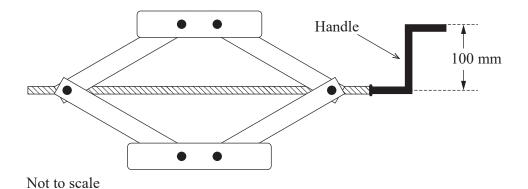
If the 2.5 mm pitch of the central screw allows the vehicle to be raised 5 mm during one revolution of the handle, the velocity ratio of the jack is
