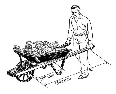
The wheelbarrow in the figure above is used by the operator to raise a 100 kg load of firewood from the ground. The weight of the load is located 500 mm from the wheel axle.
