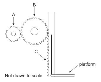
The 15-tooth gear A drives a gear train used to raise a platform a distance of 1.2 m. The teeth of gear C have a pitch of 10 mm and gear B has 30 teeth. Identify the gear train used and determine the ratio of gear A to gear C. Explain your reasoning.
