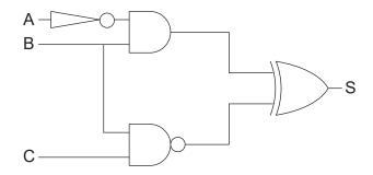
Interpret the logic circuit to create the corresponding truth table.
