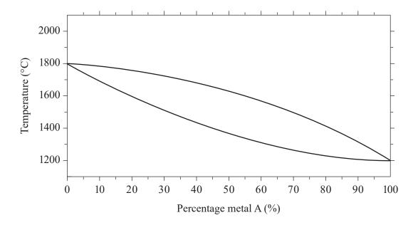
Use and annotate the binary equilibrium diagram for an alloy of metals A and B to calculate the percentage proportion of solid and liquid material present for an alloy of 50% metal A and B at 1400 °C. Answer to the nearest whole unit.
