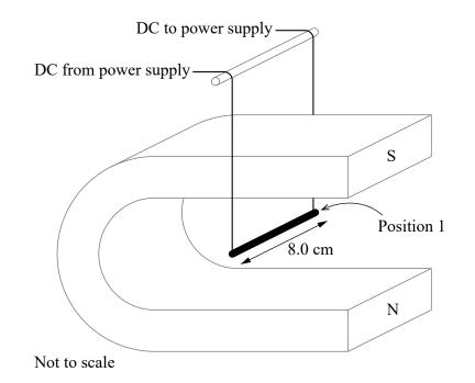
When a current (*I*) is passed through the metal rod it moves to Position 2, with an angle of  $40^{\circ}$  to the vertical.
