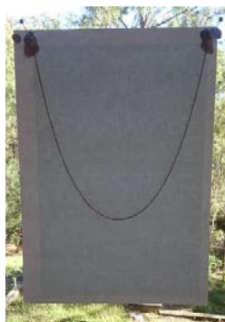
Figure 1: A photograph showing the experimental set-up with the graph paper stuck to the window and the freely hanging chain.
