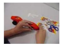
Position the screw-eyes along the centreline of the dragster body, either in front of, or behind, the axles. The screw-eyes must be parallel to the race surface. Inaccuracy will result in friction between the fishing line and the screw-eyes. Coat the screw-eye threads with a little glue. This will hold them in place.
